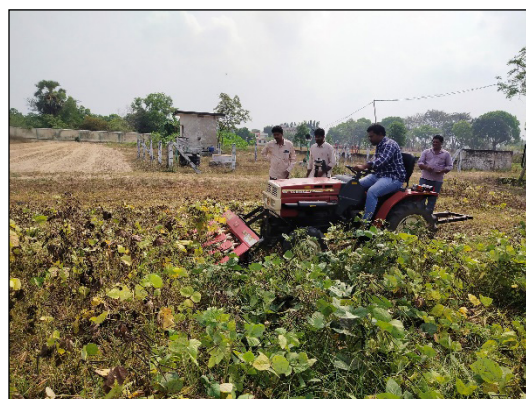
Fig. 2: Field evaluation of pulse crop harvester
