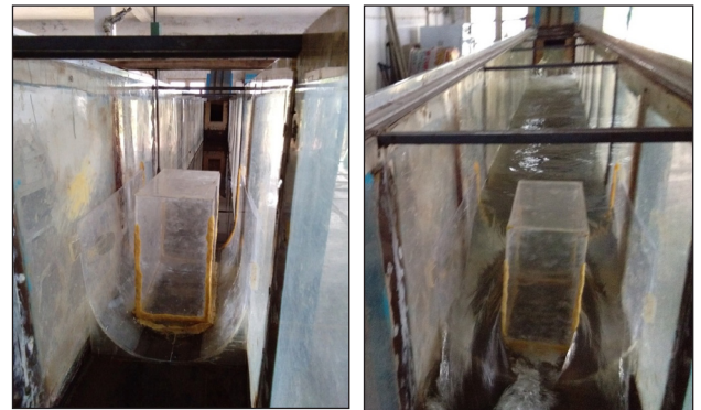
Fig. 4: Developed Circular flumes with rectangular contraction in the hydraulic flume
