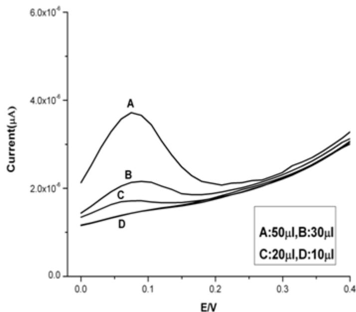
Fig. 5: Differential pulse voltograms of Star-fruit water extract in 0.1M Phosphate buffer, pH 7.0.
