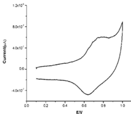
**Fig. 3:** Cyclic Voltammogram of water extract of star fruits in 0.1M Phosphate buffer at pH 7
