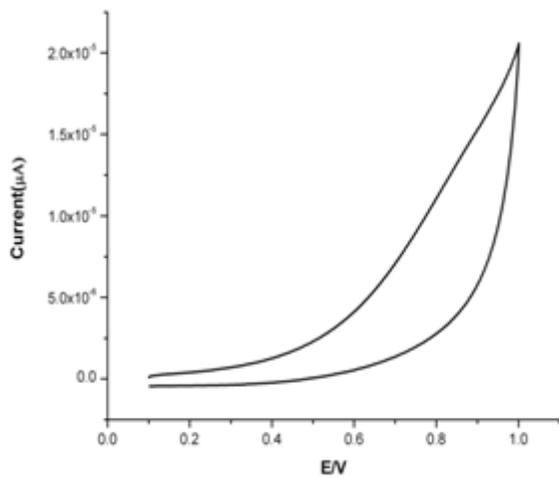
Fig. 2: Cyclic Voltammogram of Ascorbic acid in 0.1M Phosphate buffer at pH 7
