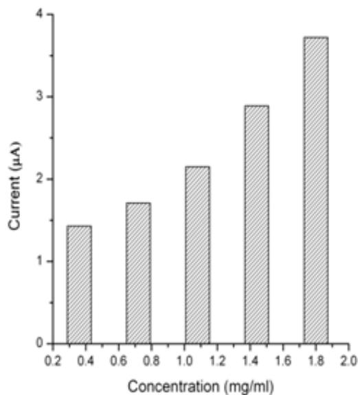
**Fig. 4:** Generation of current with different concentration of water extract of star fruit in 0.1M Phosphate buffer at pH 7 at 25°C.
