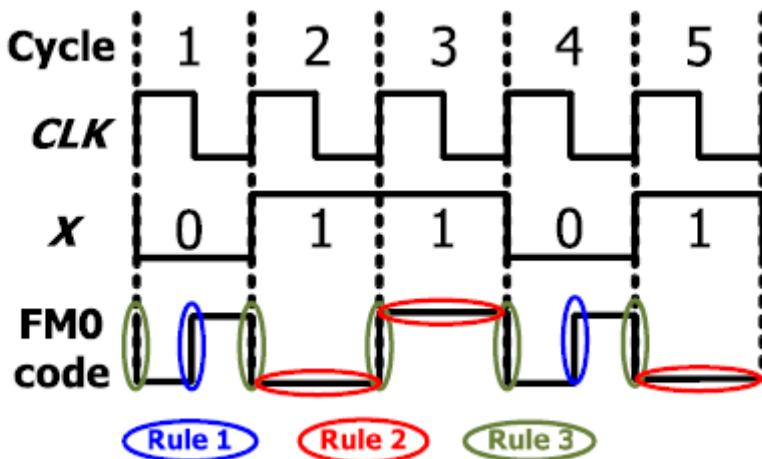
Figure 2. Illustration of FM0 coding example.
