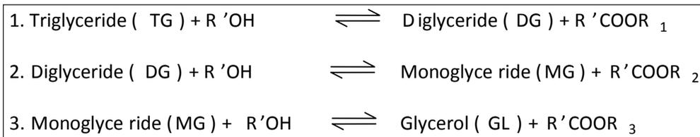
**Fig. 1:** Mechanism of transesterification reaction
