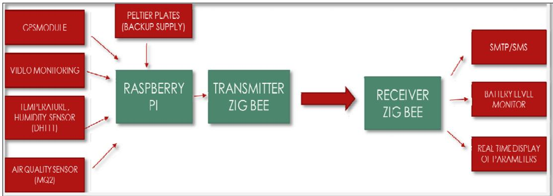
**Fig. 3:** Block diagram of proposed prototype model
