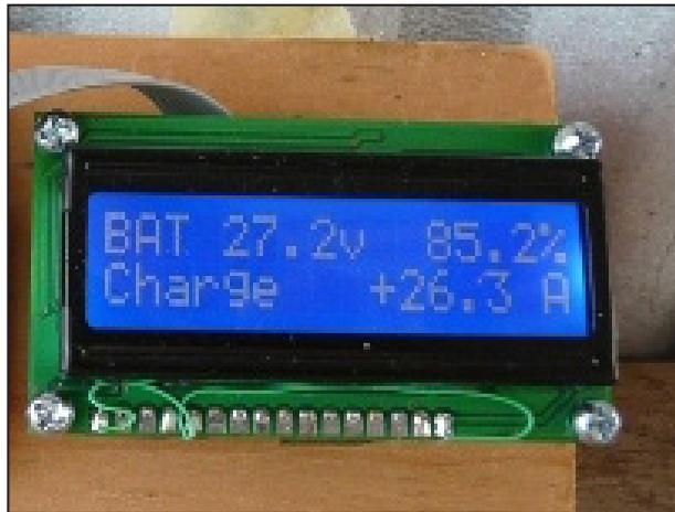
**Fig. 4:** Battery monitoring display
