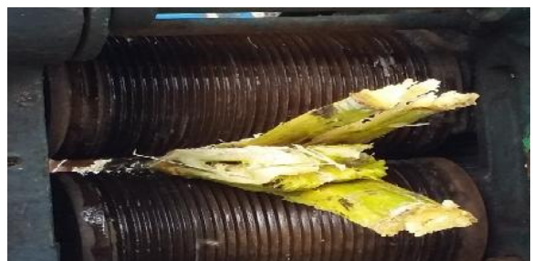
Fig. 4: 2-Roller Power Driven Sugarcane Crusher
