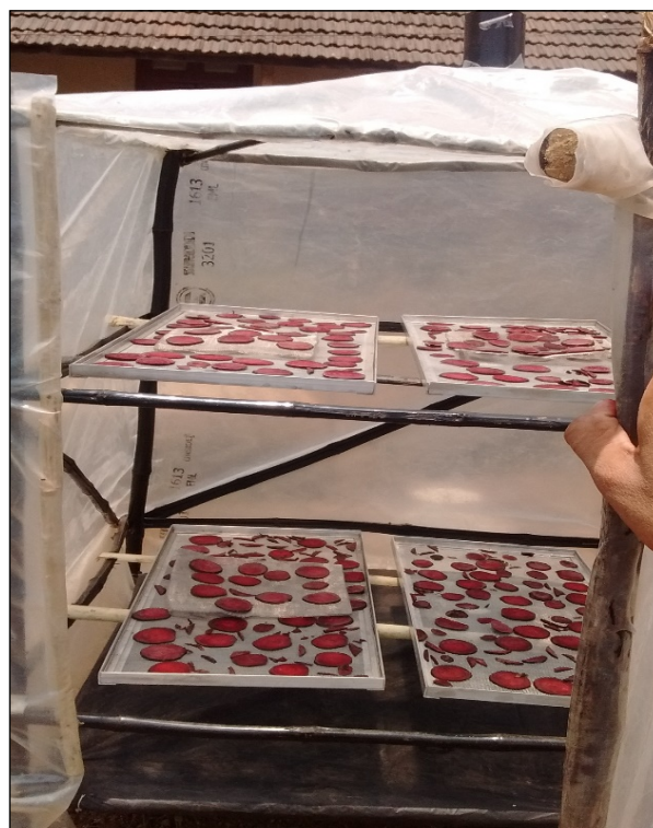
Fig. 1: Experimental setup for solar drying of beetroot slices
