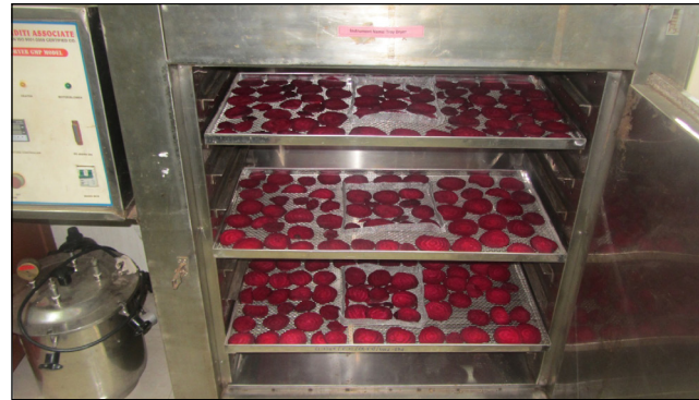
Fig. 1: Drying of beetroot slices in tray dryer & weight loss was recorded by using small perforated trays
