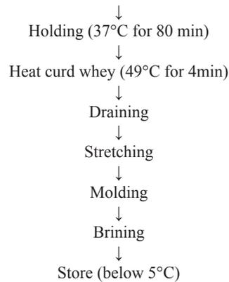
**Fig. 1:** Process flow chart for manufacturing of Mozzarella cheese by direct acidification method
