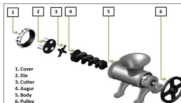
**Fig. 3:** Components of extruder type screw press briquetting machine
