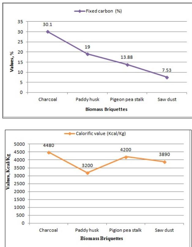
Fig. 4: Result obtained from proximate analysis of briquettes
