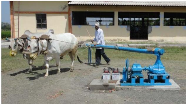
Fig. 1: Animal driven rotary mode system
