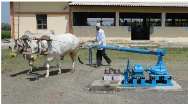
Fig. 1: Animal driven rotary mode system
