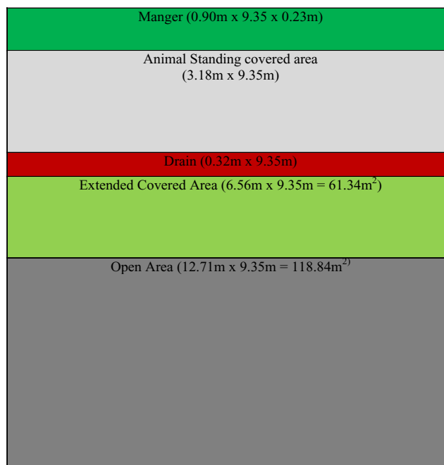
Fig. 4: Layout of Traditional Shed ( T_0 )
