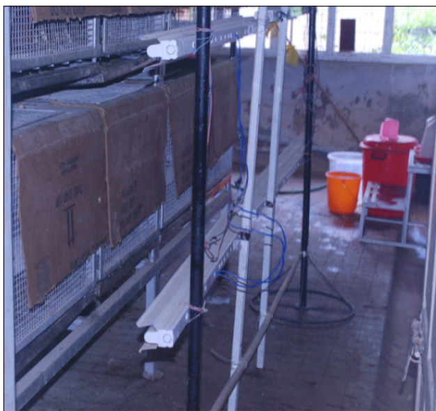
Fig. 1: UVB tubes placed in the lower front part of cages at 20 cm distance ( Source: Original)
