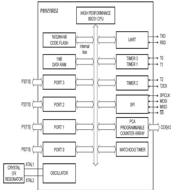
**Figure 3:** Block diagram of P89V51RD2 microcontroller.
