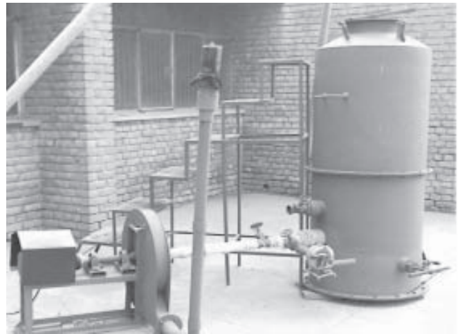
Figure 18: Imbert type downdraft gasifier of 50,000 kCal/h Capacity developed at PAU (Cost Rs 2.00 lacs)
