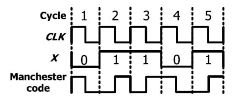
Figure 3. Illustration of Manchester coding example.
