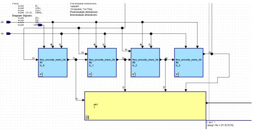
Fig 6. Block diagram of PRSG
