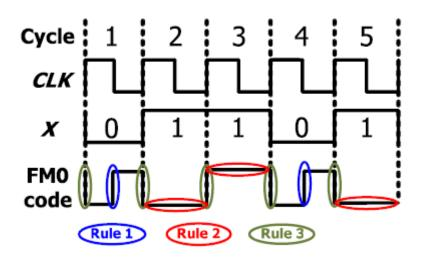
Figure 2. Illustration of FM0 coding example.
