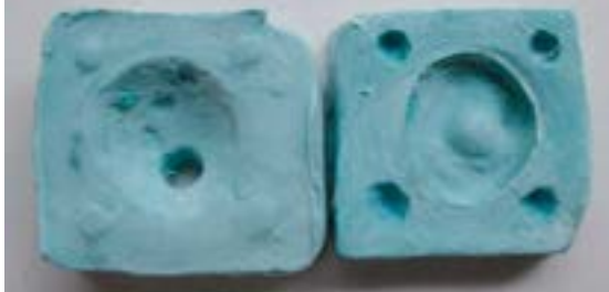
7. Mold space for wax pattern
