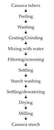
Fig. 1: Extraction of starch from cassava tubers
