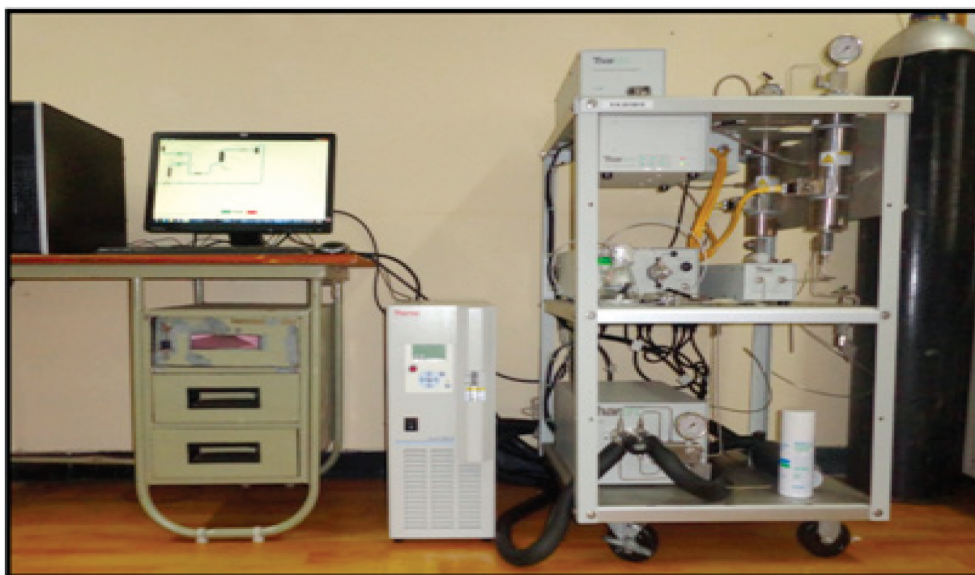
Plate 1: Experimental setup for SC- \text{CO}_2 extraction of Moringa oleifera . Lam seed kernels
