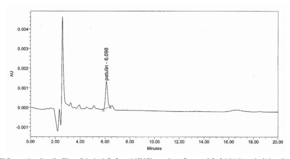
Fig. 3. HPLC separation of patulin (Waters Spherisorb  $C_{18}$ 5  $\mu$ m, 4.6 X 150mm column, flow rate: 0.5 mL/min), isocratic elution, eluent: water–acetonitrile (90:10, v/v)). Detection: UV visible; chromatogram at 276 nm
