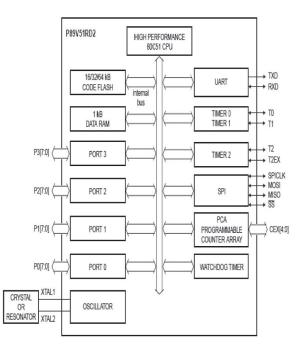
Figure 3: Block diagram of P89V51RD2 microcontroller.
