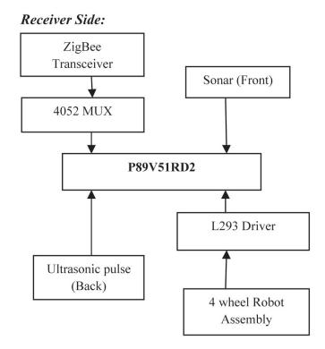
Figure 1: Block diagram of accelerometer based robot motion and speed control with obstacle detection
