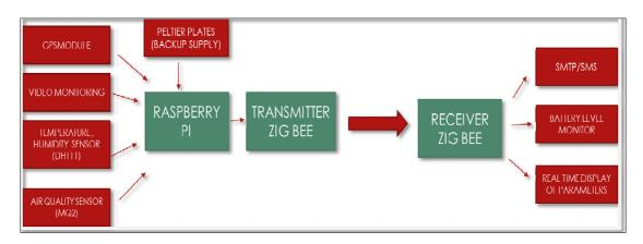
Fig. 3: Block diagram of proposed prototype model
