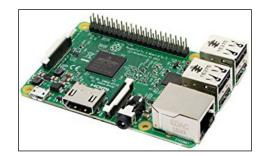
Fig. 2: Raspberry Pi Development Board
