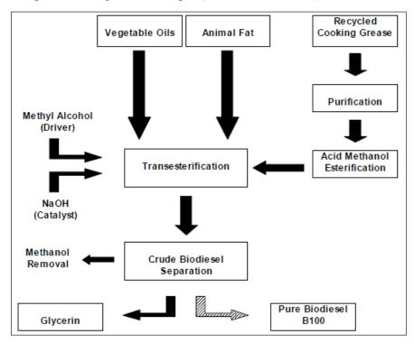
Fig. 2: Basic overview of manufacturing biodiesel
