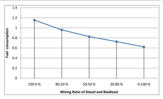
Fig. 3: Effect of diesel and biodiesel combination on fuel consumption
