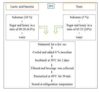
Fig. 1: Preparation of fermented linseed beverage
