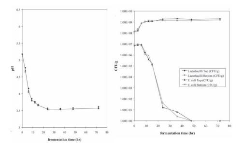
**Figure 11:** pH development in fermenting whole grain Tef flour slurry with 10% back-slopping
