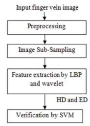
Figure 1: Process flow diagram
