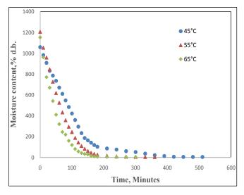
**Fig. 1:** Moisture content % (d.b.) versus time (min) of spinach leaves drying by convective hot air drying at different temperature
