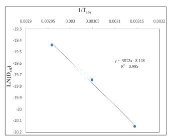
**Fig. 5:** Ln(D<sub>eff</sub>) vs 1/T<sub>abs</sub> for drying of spinach leaves dried by convective hot air drying method at different temperatures
