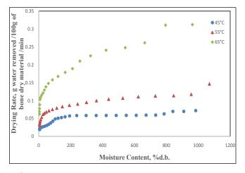
**Fig. 2:** Drying rate (g water removed/100 g of bone dry material/min) versus moisture content % (db) of spinach leaves dried by convective hot air drying at different drying temperature
