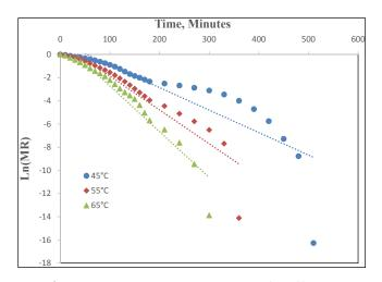
**Fig. 4:** Ln(MR) versus time, minutes for effective diffusivity for convective hot air dried spinach leaves at varied temperature
