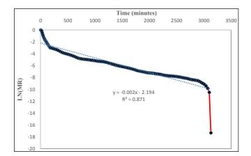
**Fig. 6:** LN(MR) versus time, min for effective diffusivity of sun dried beetroot slices
