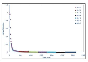
**Fig. 3:** Variation in moisture ratio with respect to time, min for beetroot slices during open air sun drying
