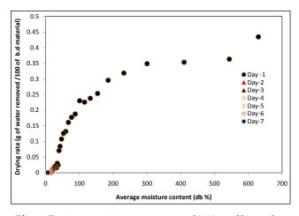
**Fig. 2:** Drying rate (g water removed/100 g of bone dry material/min) versus moisture content % (db) of beetroot slices dried by open sun drying
