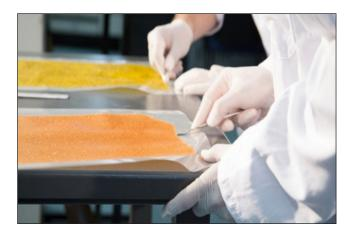
Fig. 20: Solvent casting
