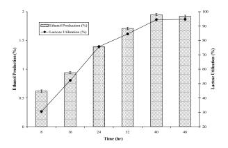
Figure 7. Effect of time on ethanol production and lactose utilization from whey using K. marxianus WIG 2
