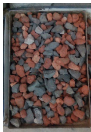
Figure-3: Appearance of Over-burnt bricks
