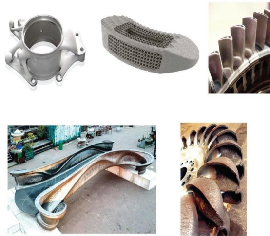
Figure 5: Applications of WAAM [28,29,30]
