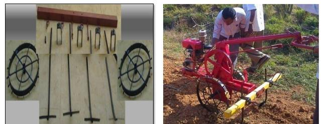
Fig. 2: Disassembled (left) and assembled view (right) of mechanical weeder
