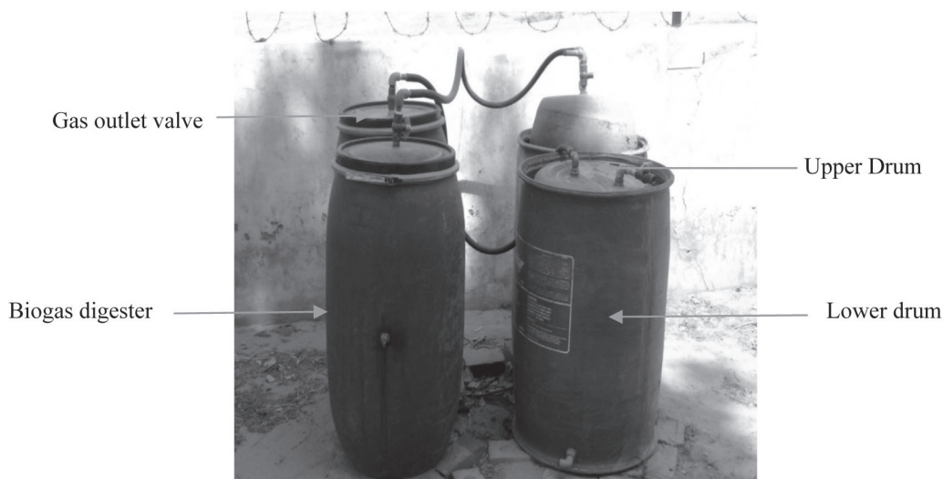
Fig. 1: Two sets of biogas digesters (124 litre capacity) along with displacement drums
