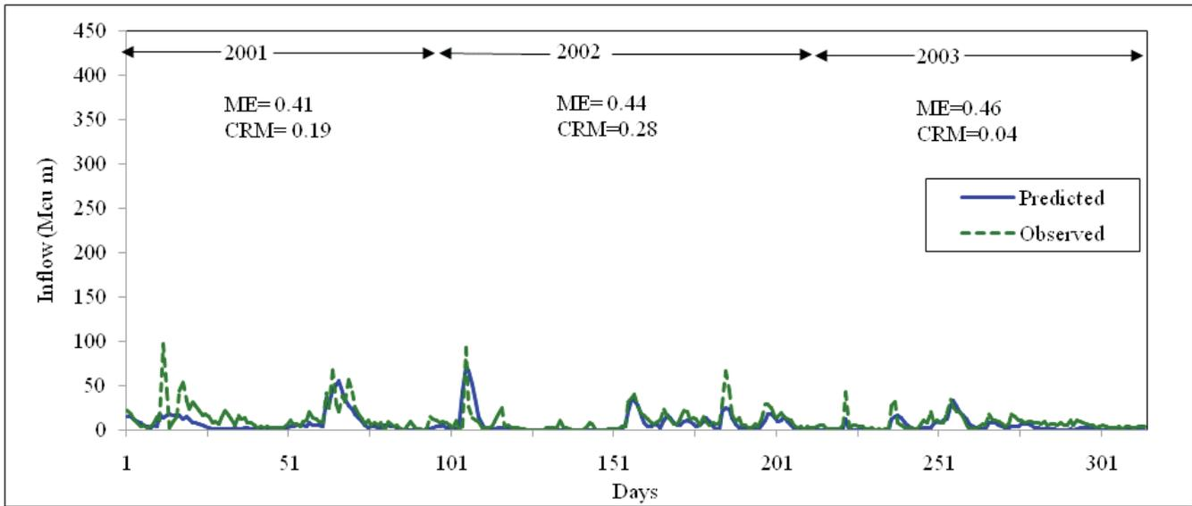
Figure 3. Time series plot for SCS CN method (validation years 2001-2003)
