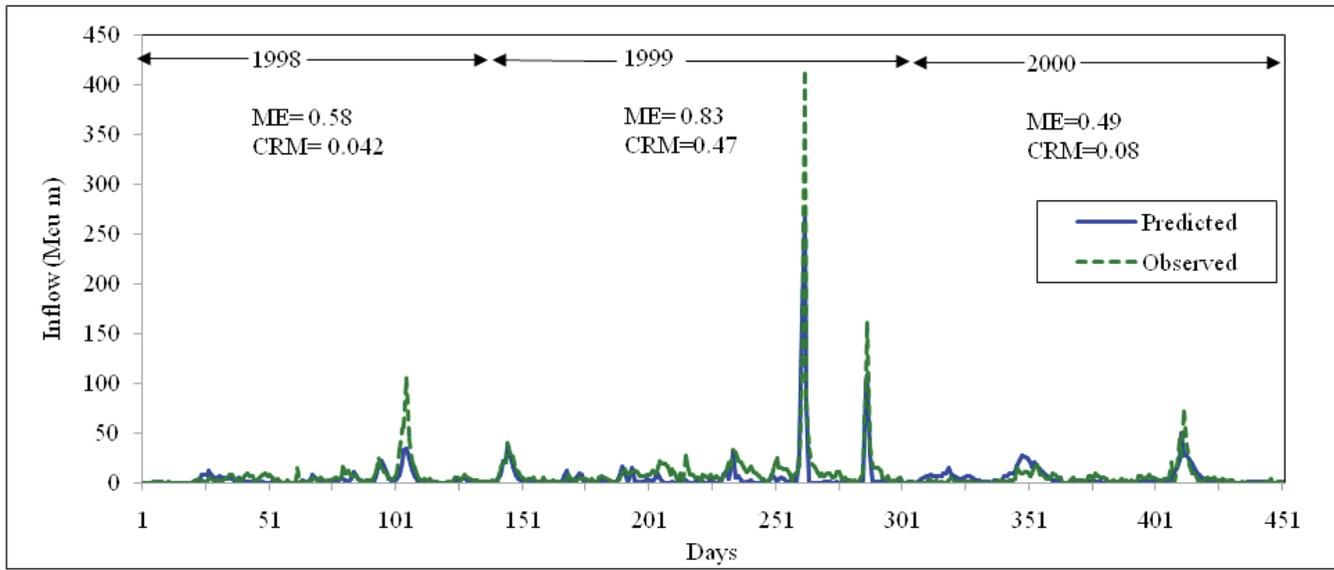
Figure 2. Time series plot for SCS CN method (calibration years 1998-2000)
