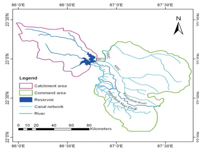
Figure 1. Catchment, reservoir and command area of Kangsabati irrigation project
