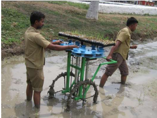
Fig. 8. Field evaluation of plug type rice transplanter
