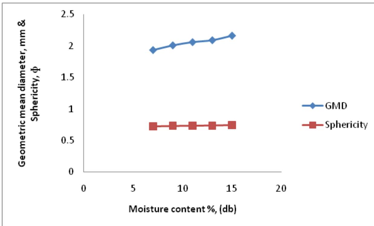
Figure 2. Effect of moisture content on geometric mean diameter and sphericity of onion seeds
