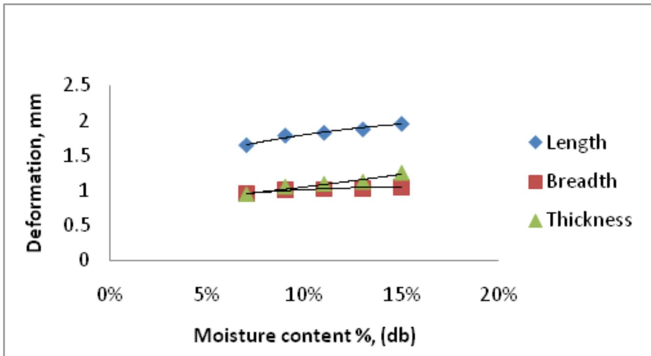
Figure 7. Effect of moisture content on deformation
