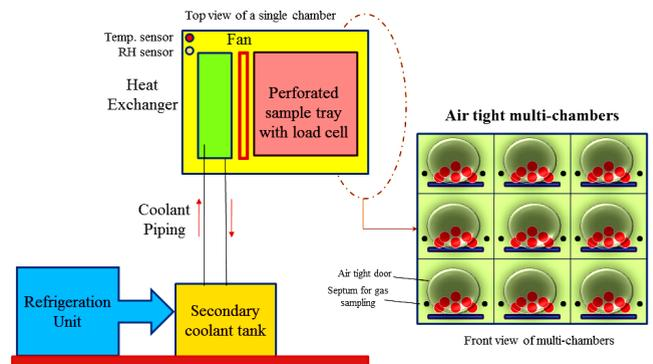
Fig. 1: Air tight multi-chamber temperature and RH control system
