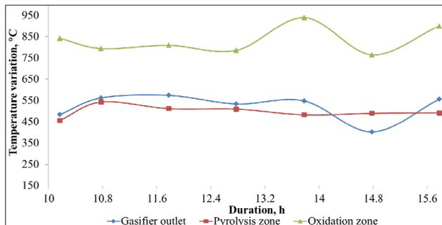
Fig. 4: Temperature variation in the reactor
