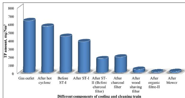
Fig. 6: Trend of TP observed in the cooling and cleaning train
