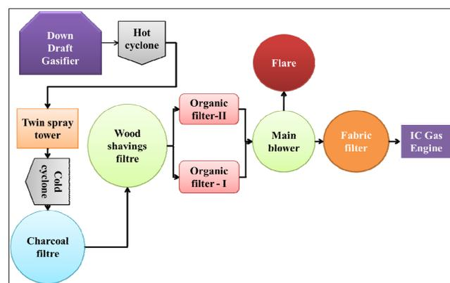
Fig. 1: Schematic of biomass gasifier with cleaning and cooling unit
