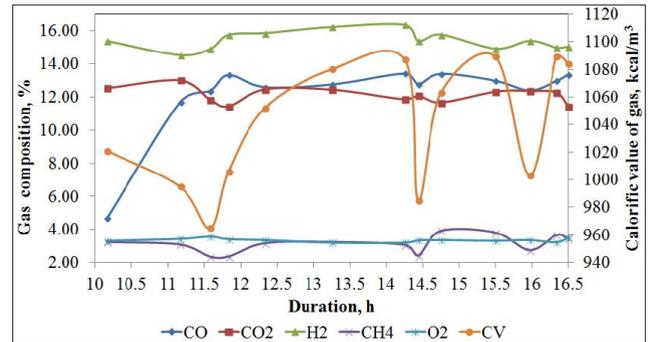
**Fig 3:** Variation in producer gas compositions and calorific value with duration
