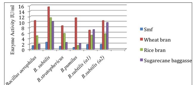
**Fig. 3:** Quantity of xylanase produced in Submerged Fermentation and Solid State fermentation
