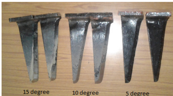
Fig. 2: Vertical rotary tiller blade's rake angle
