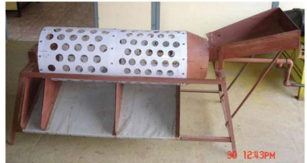
Fig. 1: (a) Rotary drum grader
