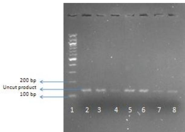
**Fig. 1: PCR-RFLP analysis on 2.5% agarose gel electrophoresis of *FecB* gene in Dorper sheep**
