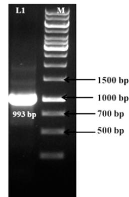
**Fig. 2:** 1% Agarose gel electrophoresis of PCR product of *trxB* amplified from genomic DNA of *Salmonella* Typhimurium strain E2375. M: 1 kb Plus ladder; L1: PCR product
