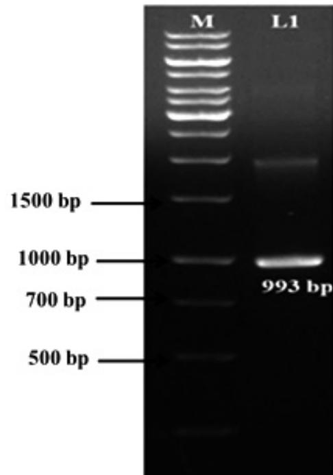
**Fig. 6.** 1% Agarose gel electrophoresis of PCR product using recombinant pET-28c(+) as template. M: 1 kb plus ladder; L1: PCR amplified product.
