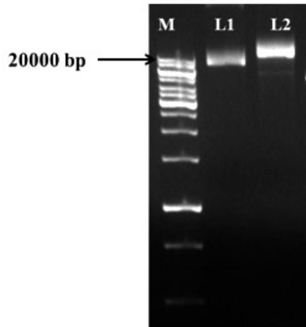
**Fig. 5.** 0.8% Agarose gel electrophoresis of un-cloned pET-28c(+) and *trxB* cloned pET-28c(+) plasmids. M: 1 kb Plus ladder; L1: un-cloned pET-28c(+); L2: *trxB* cloned pET-28c(+)
