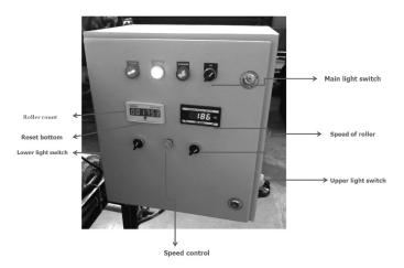
Fig. 5: Control panel of inspection table
