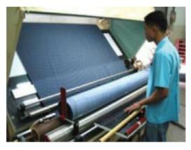
Fig. 2: Modern manual fabric inspection table.
