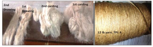
Fig. 3: TPI: 4; Count: 12 lbs/spy; Gauge length = 500 mm; Speed = 300 mm/min
