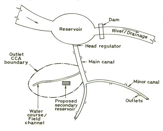
Fig. 1 Definition sketch of the proposed secondary reservoir in the surface irrigation project
