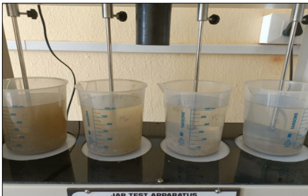
Fig. 2: Jar test apparatus for treatment of turbid water by biocoagulants
