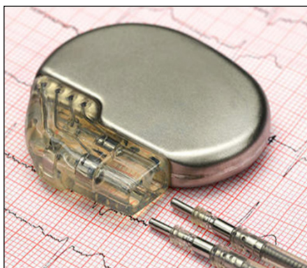
Fig. 1: Pacemaker generator with lead
