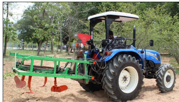
Fig. 1: Developed tractor operated basin making cum fertilizer applicator
